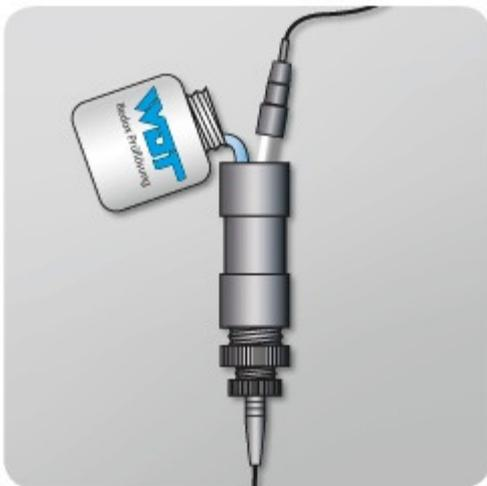
1. Screw out the ½" platinum electrode from the bottom of the measuring cell, depose the blue beads on absorbent paper.
