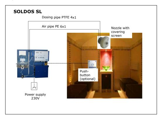
We recommend to install the hose pipe for the brine solution and for the the compressed air in a standard empty conduit d20.
