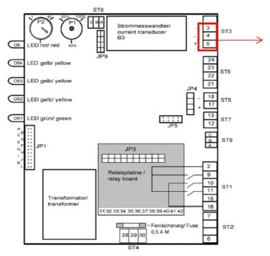
The WDT steam performance controller has to be connected to the connectors 3, 4 and 5 of the Hygromatik controller.
